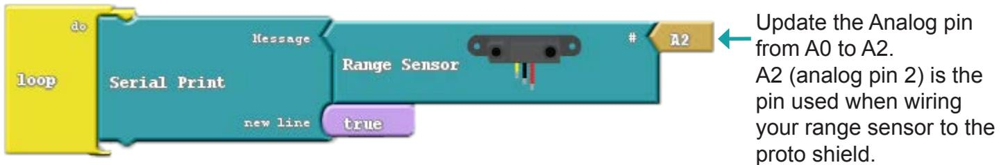
Now that you have your programming block setup, **make sure your Arduino is plugged in and turn off the battery pack** and press the **Upload to Arduino** button. After compilation, the Arduino IDE will upload the data to the Arduino.
