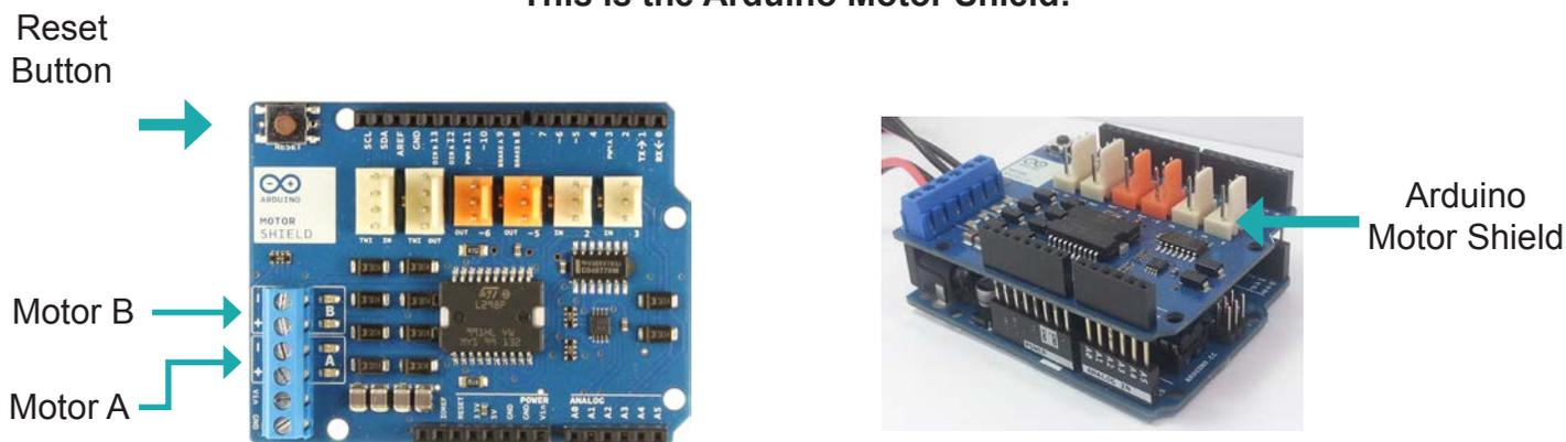
The motor shield is what allows our Arduino to control motors relatively easily without having to worry about too much extra wiring or extra components.
